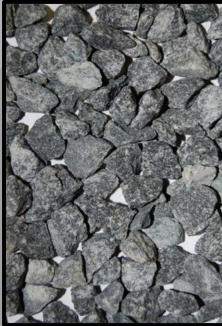
\frac{3}{8} -inch Single Size, Cubical, and Durable
